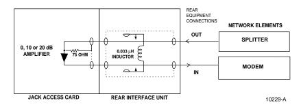
Figure 34. Typical Interconnect with Gain Application
